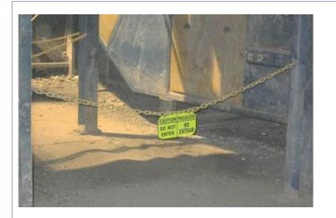
An example of a warning sign to prevent foot traffic beneath a conveyor sorting line.
