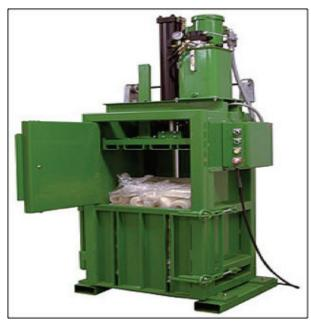
down into a dense cube, it is tied as a bale by a thick wire and then pushed out of the machine. This process allows for easy transport of all materials involved.
