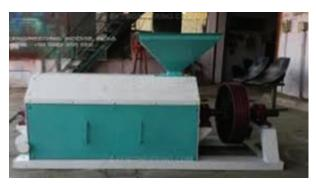
shredders tear up the plastic into small pieces/ flakes, preparing them for recycling into other products. Shredded plastic is easier to use in road construction and is the feed/raw material for the agglomeration stage. Shredder includes cutting tools welded on the shaft, connected to an AC Motor.
